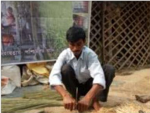
1 Cutting sticks according to length
